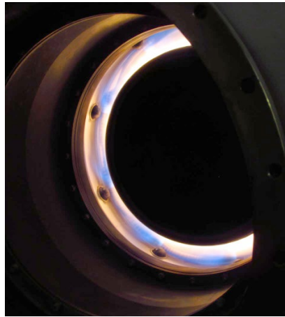
Safran's engineers have managed to stabilize the flame in a swirling gas flow, thus reducing the required number of fuel nozzles.
