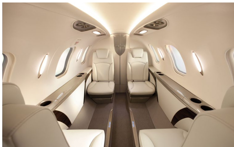
The over-the-wing engine mount design makes more room in the cabin. Honda Aircraft expects the most popular configuration to be the executive version, with leather seats and an under-seat storage drawer.
