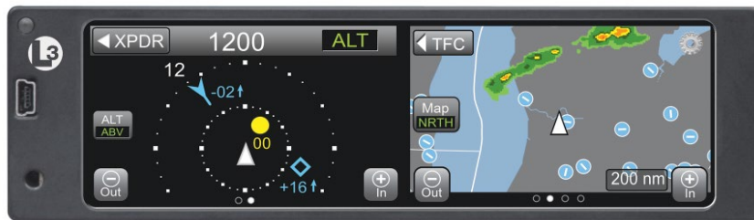
The L-3 Lynx displays both traffic and weather on its own touchscreen or pilots' devices.
