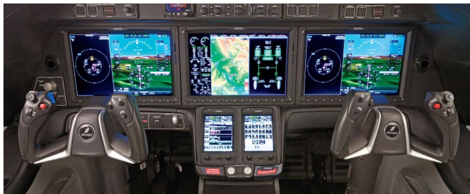
Location of the G3000's touchscreens relative to the pilot was a key concern for HondaJet designers, who wanted to find the optimal location and tilt angle to work eye-distance constraints. Avionics options include synthetic vision, radar altimeter, CPDLC, Iridium satcom, Tcas II, Taws A and Garmin SurfaceWatch.
