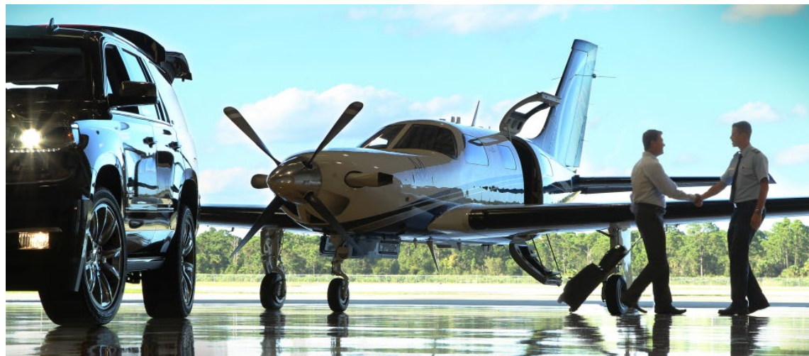
The Piper M600 has an mtow of 6,000 pounds and a range of 1,484 nm.
