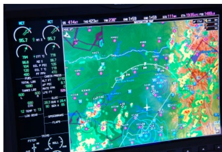
Location of the G3000's touchscreens relative to the pilot was a key concern for HondaJet designers, who wanted to find the optimal location and tilt angle to work eye-distance constraints. Avionics options include synthetic vision, radar altimeter, CPDLC, Iridium satcom, Tcas II, Taws A and Garmin SurfaceWatch.
