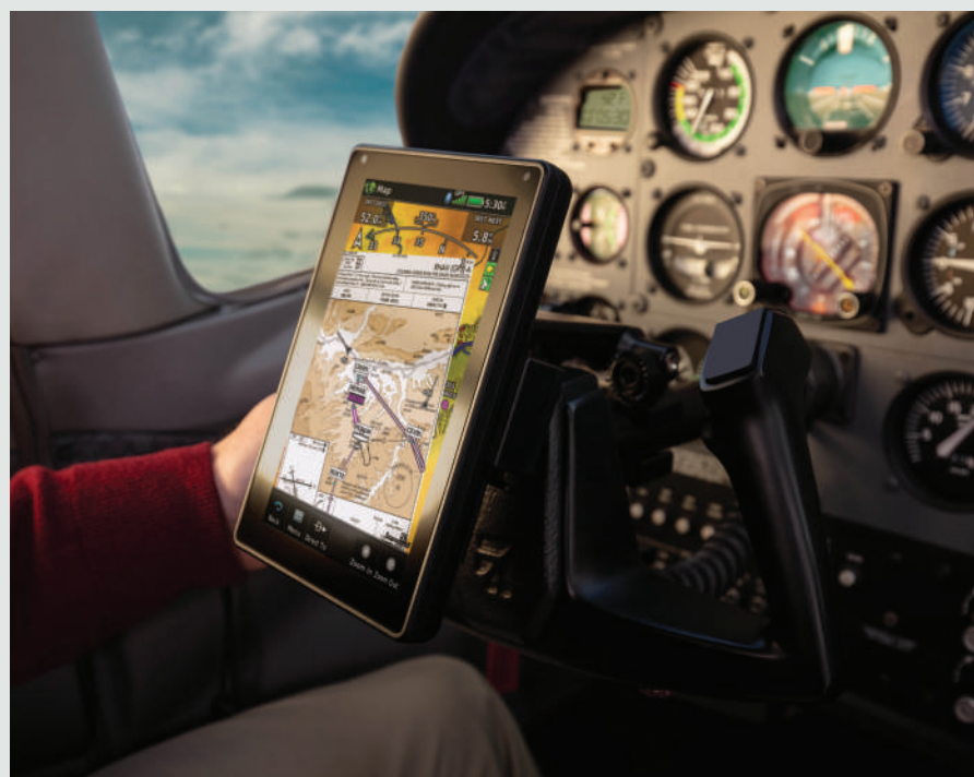
Garmin's newest portable GPS device, the aera 760, packs many features into a compact unit, including approach chart overlay, procedures in flight plans, and synthetic vision.
