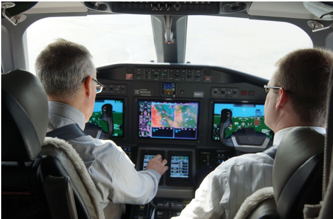
The flight deck is the same Garmin G5000 touchscreen-controlled Intrinziec system used in several other Citation models. Pilots can expect a roomy and uncluttered front office, with the center console trimmed and switches moved to the sidewall for a clean, modern feel and many fewer switches, knobs and controls for a clean, modern feel.
