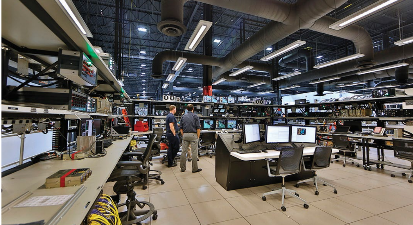
The new G500/G600 cockpit (below) includes active control sidesticks and touchscreen avionics controllers and eliminates a huge number of switches, knobs and controls. The systems integrations bench lab (left) allows engineers to wring out the airplane's digital network.
