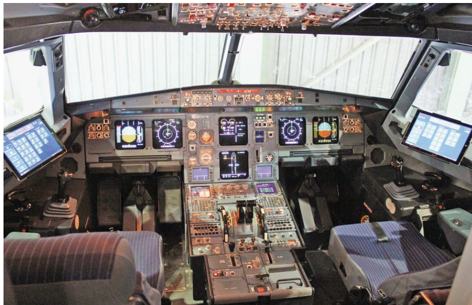
Surface Pro 3 computers mounted in an Austrian Airlines A320.
