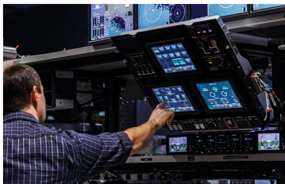
The G500 integration test facility features a flyable cockpit (above) where pilots can test all the new features such as touchscreen-controlled avionics and the new active control sidesticks. Engineers can see exactly what pilots are doing on large-screen monitors that replicate cockpit displays (right).
