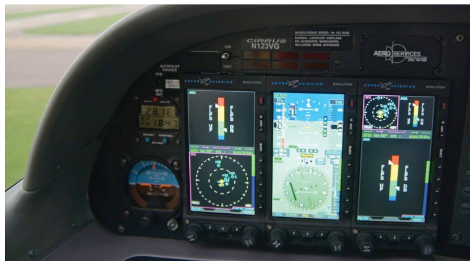
Aspen has added to its Evolution displays a software-only upgrade that provides an angle-of-attack indicator.
