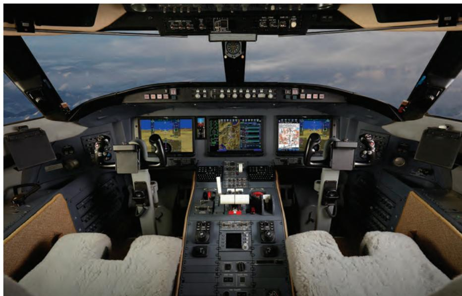
A Collins Aerospace Pro Line Fusion avionics upgrade will solve upcoming obsolescence issues facing Pro Line 4 displays and other key components on Bombardier Challenger 604s.
