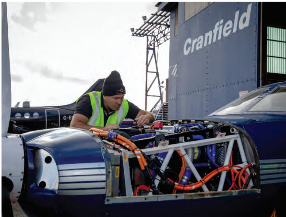
ZeroAvia's hydrogen propulsion system installed in a Piper M Series single-engine aircraft.
