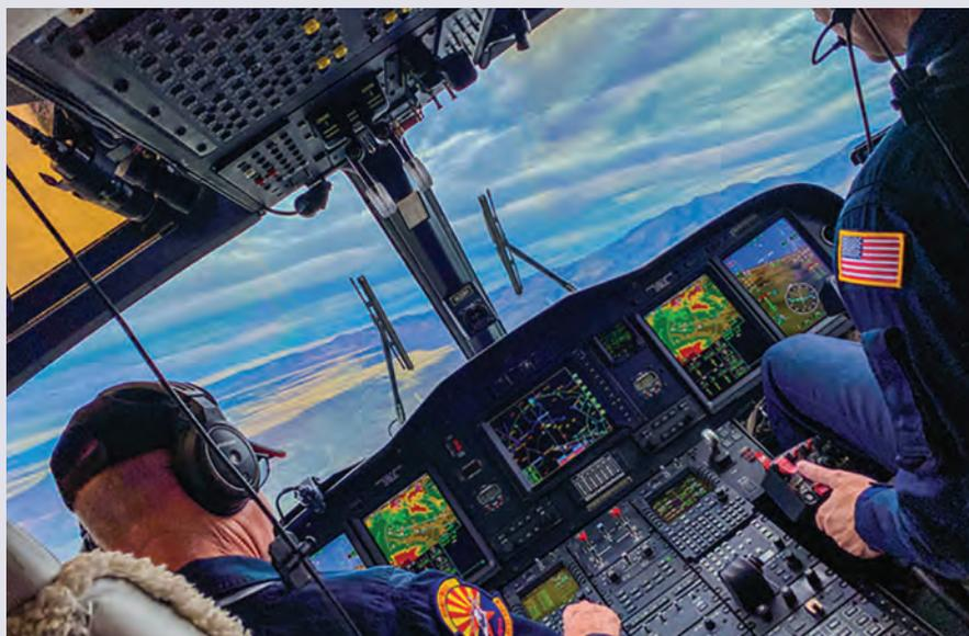
Honeywell’s Phase 8 upgrade adds track-centered synthetic vision system and new offshore instrument approach capabilities to the Leonardo AW139.
