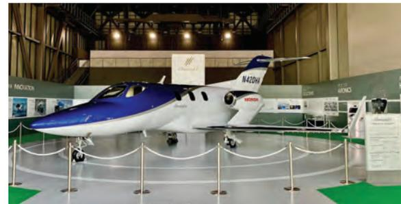
(OTWEM) design wasn’t intended to make the HondaJet look unusual, which it certainly did, but took advantage of aerodynamic optimization that delays drag rise at high speeds. Although this was confirmed in a Boeing wind tunnel, the POC flight testing proved that the concept worked. Another key benefit of OTWEM is the larger space available in the cabin by moving engine structure and systems out of the fuselage.
