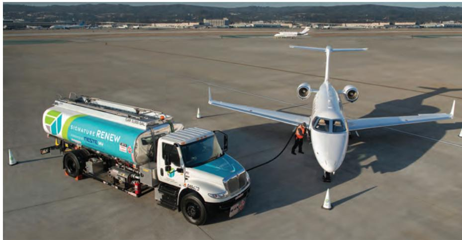
An Embraer Phenom 300 uplifts sustainable aviation fuel at the Signature Flight Support FBO in San Francisco. The Signature Renew fuel is a 30/70 blend of renewable feedstock and conventional jet-A that yields a 25 percent reduction in direct carbon output from aircraft versus traditional jet fuel.
