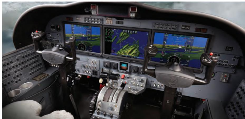
The Pro Line Fusion upgrade for the CJ2+ adds new features that include integrated V-speeds, fuel sensing, predictive performance, and controller-pilot datalink communications.
