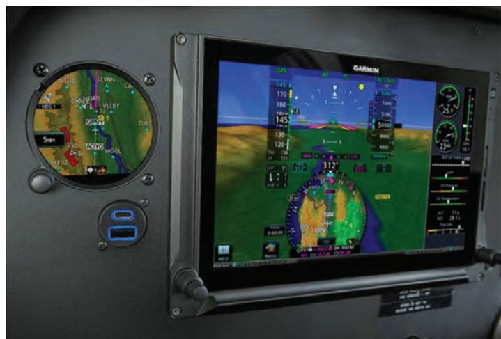
Garmin's GSB 15 chargers come with new features that include increased power output up to 27 watts per port and either dual Type-C or combined Type-C and Type A USB ports as well as short-circuit and over-temperature protection.
