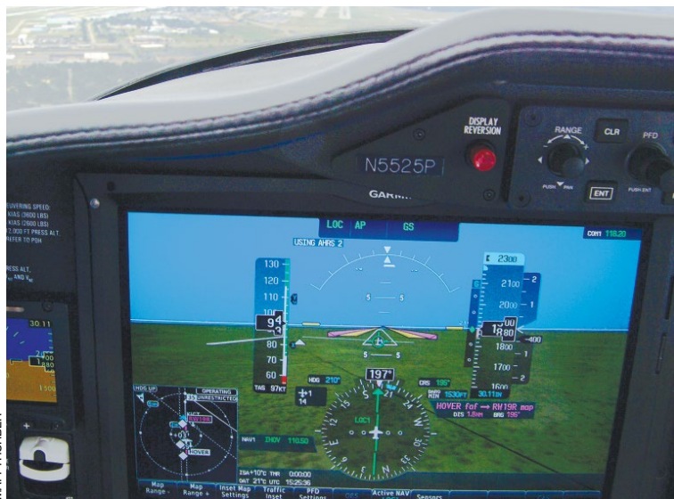
On final approach on the ILS Runway 19L at Wichita's Dwight D. Eisenhower National Airport. The Garmin G2000's automatic flight control system smoothly manages the approach, depicted on the PFD's synthetic vision display.
