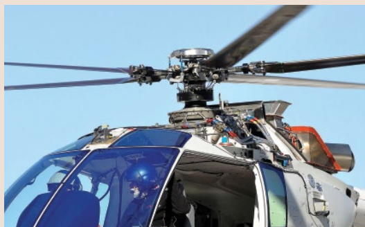
Marengo has redesigned the SKYe SH09's main rotor head to reduce vibration and complexity, while enhancing its adaptability to accept future upgrades.
