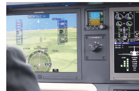
To prepare for the steep approach we flew a 5.5-degree approach with autobrakes set.
