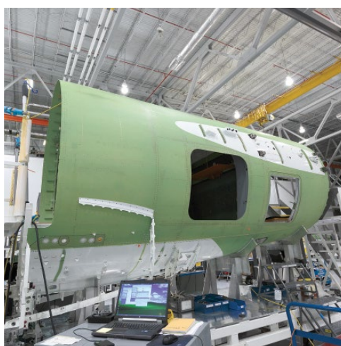
The airframer's Savannah campus includes two 400,000-sq-ft factories for production of the in-development G500 and G600. The company uses one of the factories for wing and tail construction, activities it brought in house for these aircraft, and the other for fuselage production and final assembly. G500 shown here.
