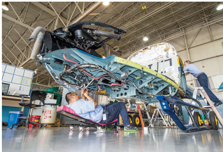
An AS350BA AStar belonging to the Lee County Sheriff's Office recently underwent a 12-year inspection at the Airbus Helicopters Grand Prairie, Texas facility. It is the second such inspection for that helicopter.
