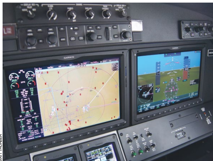
The Garmin 3000 is well suited for single-pilot operations, and the pilot can reach the touchscreen controls from either seat. The trimmed-down center console houses the power levers, flaps lever and trim controls.
