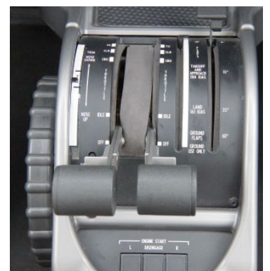
The Garmin 3000 is well suited for single-pilot operations, and the pilot can reach the touchscreen controls from either seat. The trimmed-down center console houses the power levers, flaps lever and trim controls.
