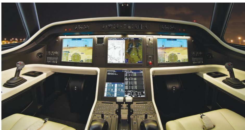
Like the larger Legacy 500, the 450 features a fly-by-wire Rockwell Collins Pro Line Fusion flight deck. The front office has an uncluttered feel, as sidesticks take the place of conventional ram's horn yokes.
