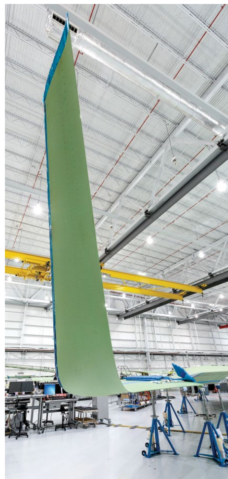
The airframer's Savannah campus includes two 400,000-sq-ft factories for production of the in-development G500 and G600. The company uses one of the factories for wing and tail construction, activities it brought in house for these aircraft, and the other for fuselage production and final assembly. G500 shown here.
