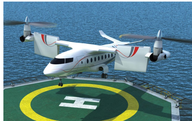
AgustaWestland is planning to fly its next-generation civil tiltrotor in 2021. The 20-passenger rotorcraft, which is much larger than the in-development nine-seat AW609 tiltrotor, is now in the conceptual design phase.
