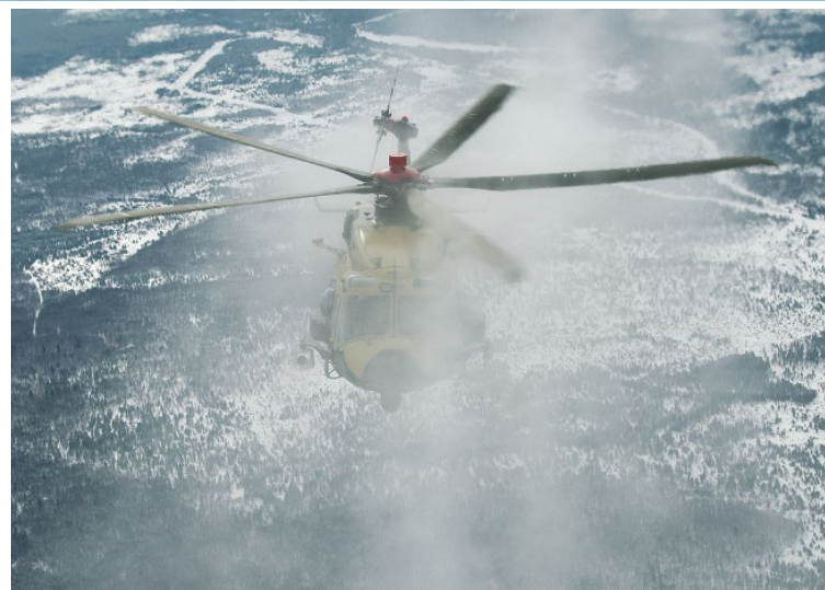
AgustaWestland will continue icing trials on the AW189 this winter, as it pursues certification of the full icing protection system. Certified in 2014, the helicopter is currently equipped with a limited icing protection system.
