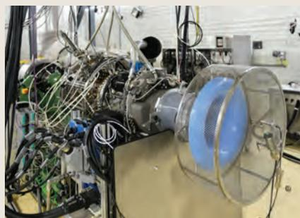
test bench for turbomachinery combustion and aerothermal testing located at the company's facility in Bordes, France.
