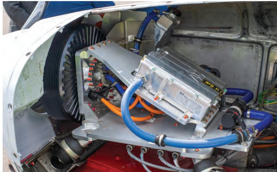
With its Electric EEL technology demonstrator Ampaire is developing a hybrid-electric propulsion system to convert existing regional airliners.
