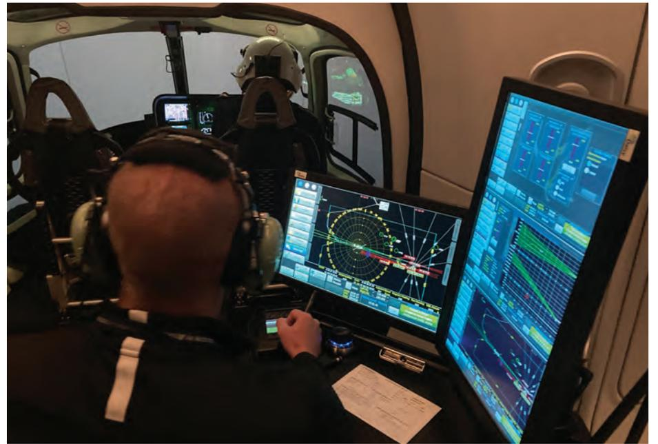
Air Methods trains its pilots how to handle inadvertent flight into instrument meteorological conditions in a FlightSafety simulator, as part of the helicopter operator's SMS efforts.
