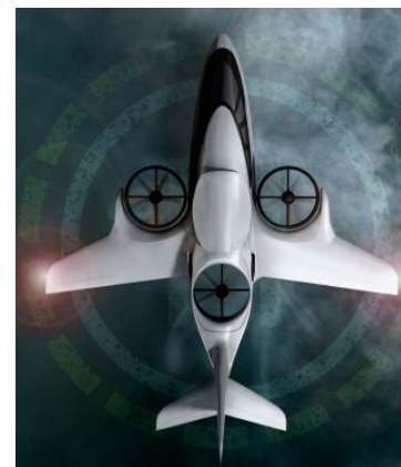
The TriFan 600's aft-mounted third fan is stowed during cruise, while the wing-mounted fans rotate
