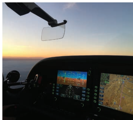
The low-cost SkyDisplay HUD brings added safety and utility to smaller aircraft.
