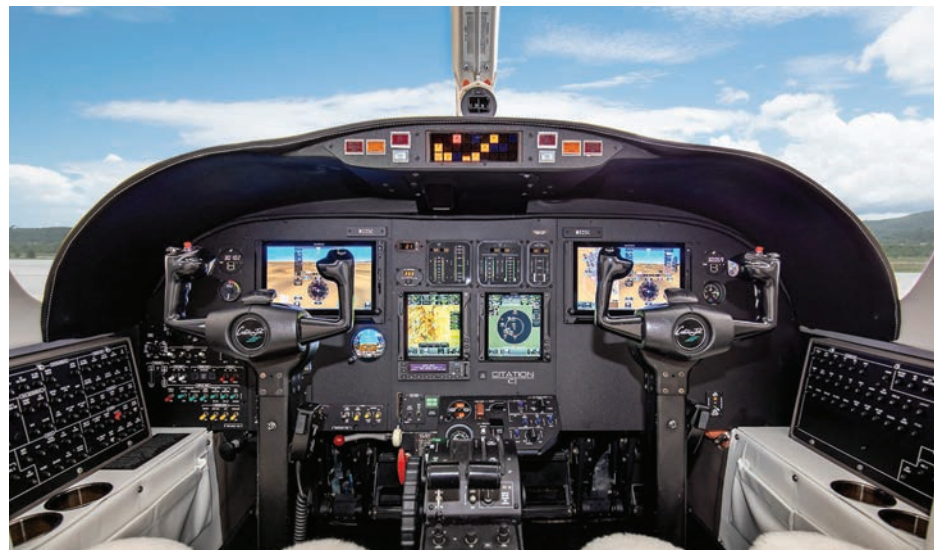
JetTech's new supplemental type certificate provides Garmin cockpit avionics upgrade solutions for Cessna CitationJets through S/N 0359.
