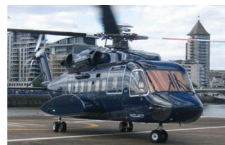
(Top) While attempting to land at a private landing site, the pilots flying a Sikorsky S-92 descended to 28 feet agl before initiating a go-around then successfully landing. (Right) The S-92 operated by Starspeed Ltd. had to undergo a series of maintenance inspections in Stansted due to overlimiting the engines, with torque reaching 131 percent during a go-around.
