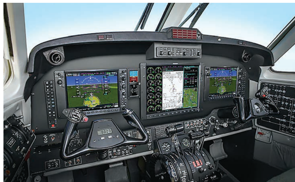
Garmin's G1000 NXi suite installed in a Blackhawk Aerospace Technologies-modified King Air.
