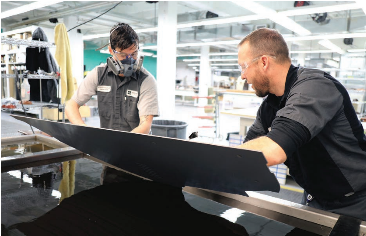
Duncan Aviation has developed new capabilities for hydrodipping large components such as table inserts or galley tops. A film-transfer process, hydrodipping costs much less and is more sustainable than traditional treatments for wood and other cabin interior materials.
