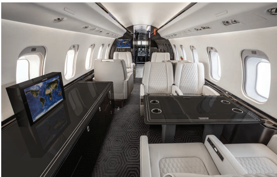
This credenza top and card table are finished using Duncan Aviation’s hydrodipping process, which replicates surfaces that look like the real materials.
