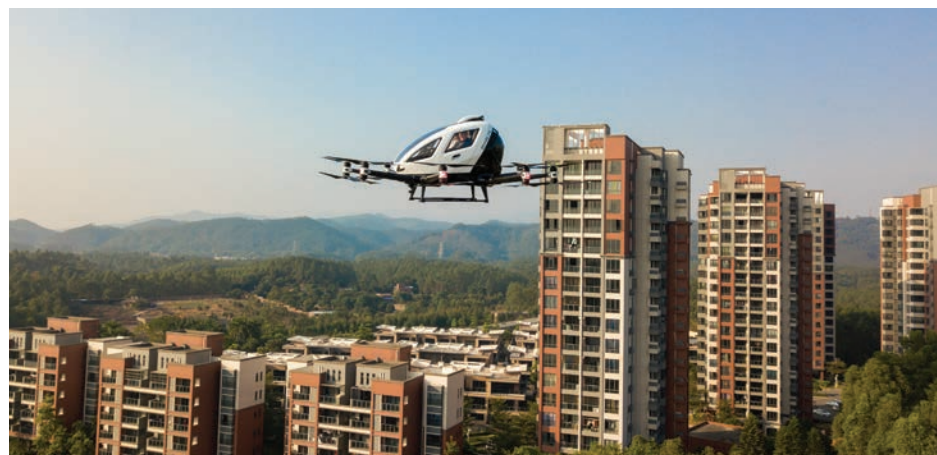
EHang’s all-electric, fully autonomous EH216 eVTOL aircraft is being developed for short flights carrying passengers and for a variety of applications including logistics and fire-fighting.
