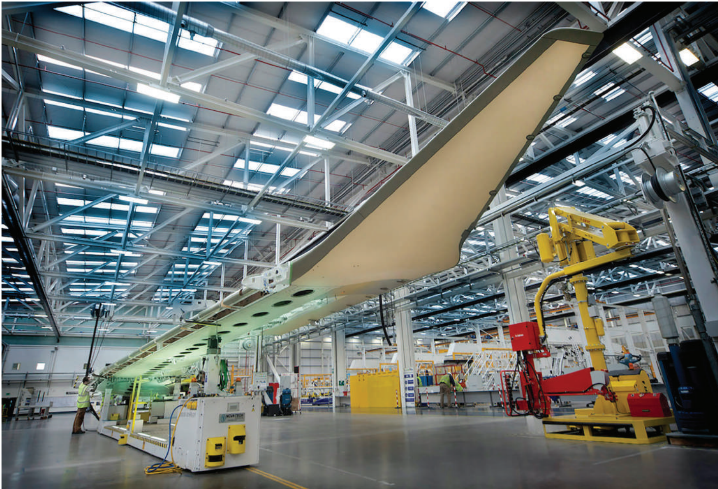
Bombardier UK manufactures composite Airbus A220 wing assemblies at its plant in Belfast, Northern Ireland, using the sophisticated resin transfer injection process—a first for commercial aircraft wing manufacturing.
