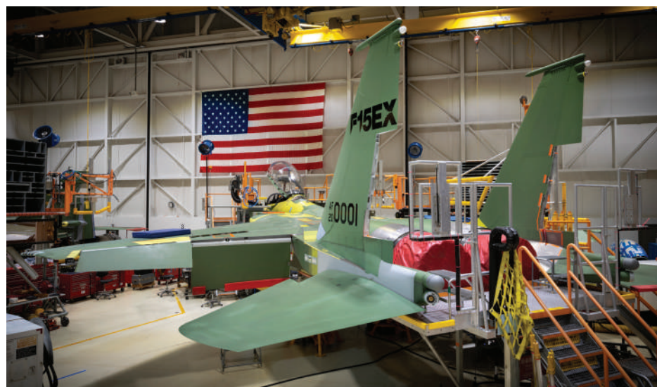
The first F-15EX takes shape in the St. Louis factory. It wears the Air Force serial 20-0001.
