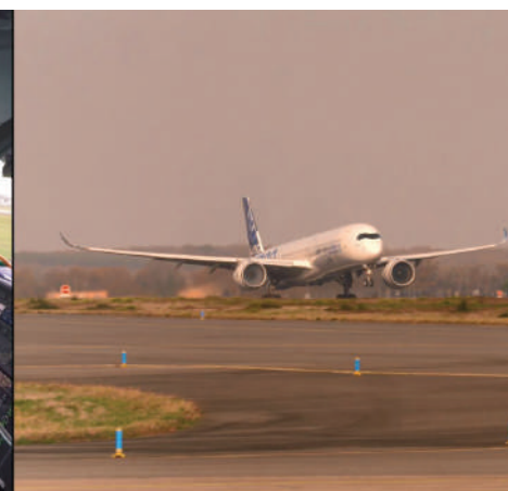
Airbus's ATTOL project achieved several fully autonomous flights in which an A350 widebody taxied, took off, and landed without intervention by pilots in the flight deck.
