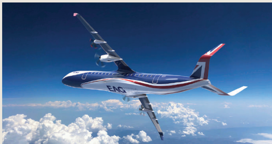
Electric Aviation Group says its HERA airliner will carry 70 passengers up to around 800 nm.
