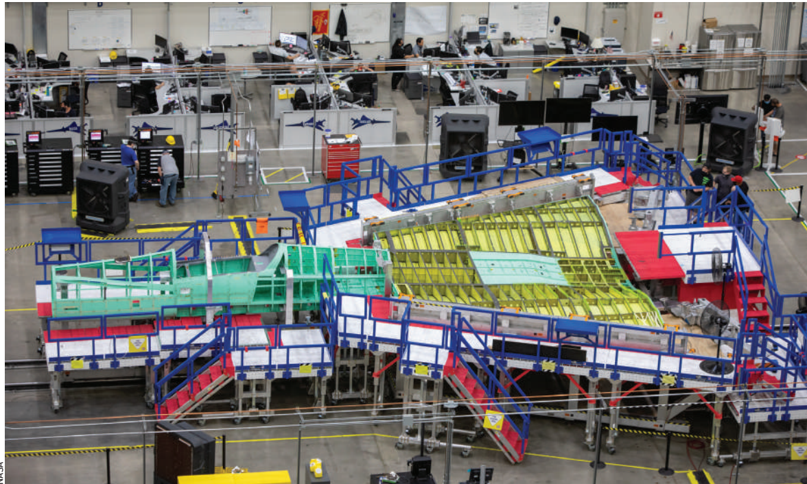
Assembly of the wing and forward section of the NASA/Lockheed Martin X-59 Quiet SuperSonic Technology (QueSST) demonstrator is underway as NASA strives to demonstrate the feasibility of quiet supersonic travel over land.
