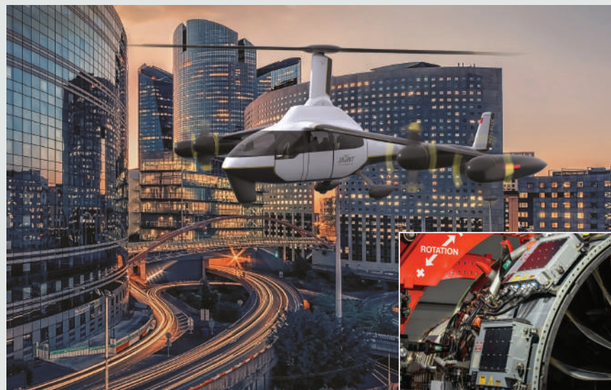
BAE Systems is working to produce control systems for new electric aircraft like Jaunt Air Mobility's planned family of eVTOL models. The systems need to be far smaller and lighter than the unit shown (inset) on a conventional turbofan engine.
