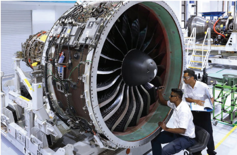
Engineers at the Pratt & Whitney-SIA Engineering MRO joint venture Eagle Services Asia in Singapore inspect a newly overhauled PW1100G.
