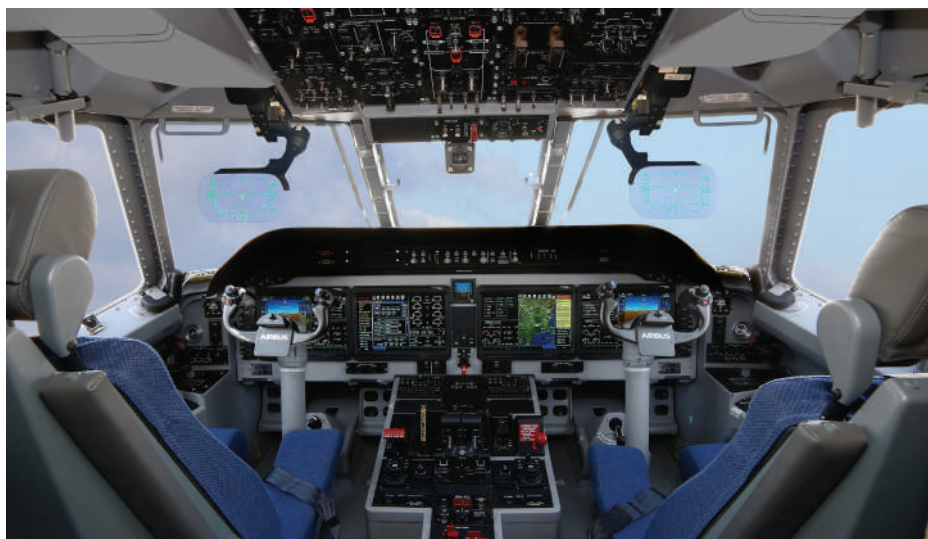
Collins Aerospace’s Pro Line Fusion avionics appears on the flight deck of an Airbus C295 tactical airlifter. Collins is turning to more defense work as a way to offset a decline in its commercial aviation business.
