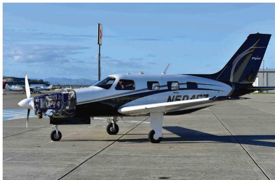
Hydrogen propulsion system pioneer ZeroAvia has been flight-testing a converted Piper M600 piston single and has laid plans to power larger aircraft in the future.
