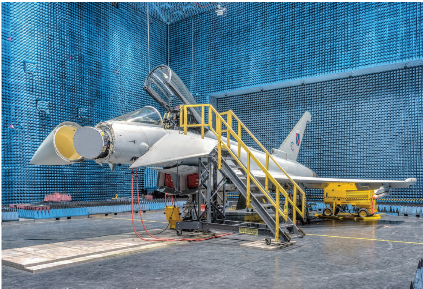
The Eurofighter Typhoon trials aircraft—IPA5—with the Captor-E radar undergoes tests in an anechoic chamber.
