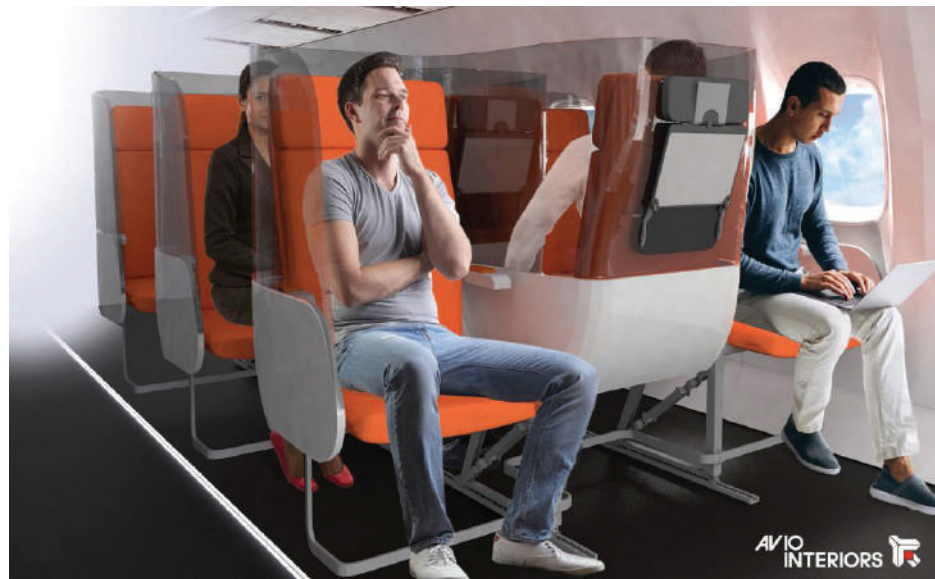
AvioInteriors' Janus concept features a center seat of a three-abreast layout positioned in the opposite direction from those on the aisle and next to windows.
