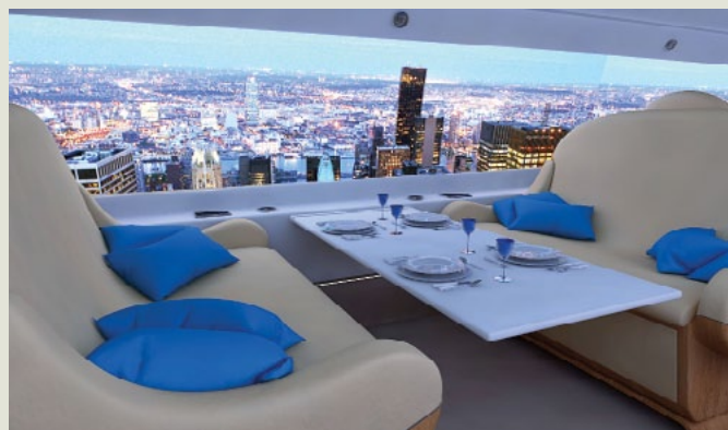
The cabin of the future might not have windows if Spike Aerospace's plan to eliminate windows to reduce weight and lower drag in its supersonic jet gains traction in the larger market.
