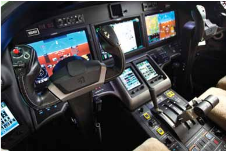
The Garmin G5000 flight deck replaces the Honeywell Primus Epic avionics in the new Citation Sovereign. The touchscreen interface removes the buttons and knobs for a cleaner look, but there is a rotary knob for pilots who prefer that format.
