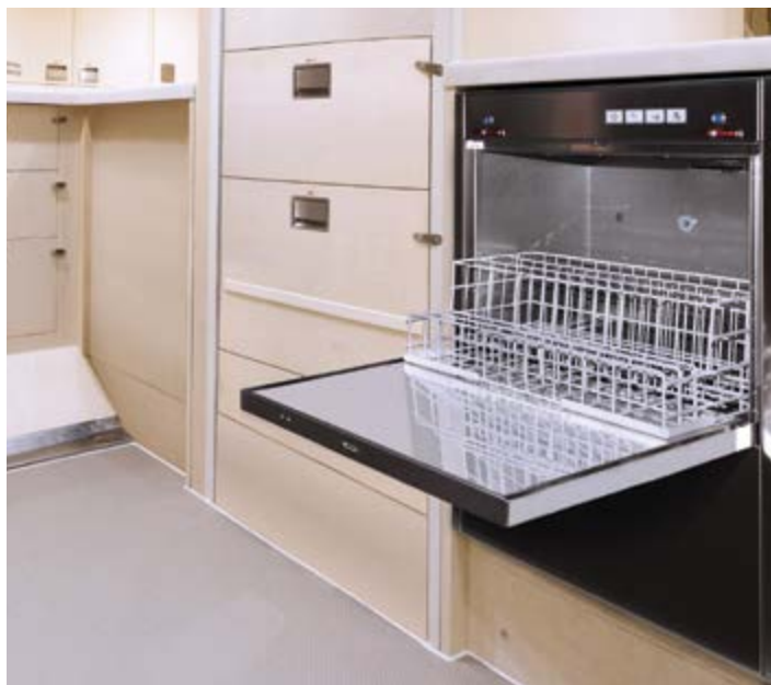
Jet Aviation Basel has developed for widebody aircraft a plug-and-play in-flight dishwasher with a three-minute wash cycle that runs on three liters of water.
