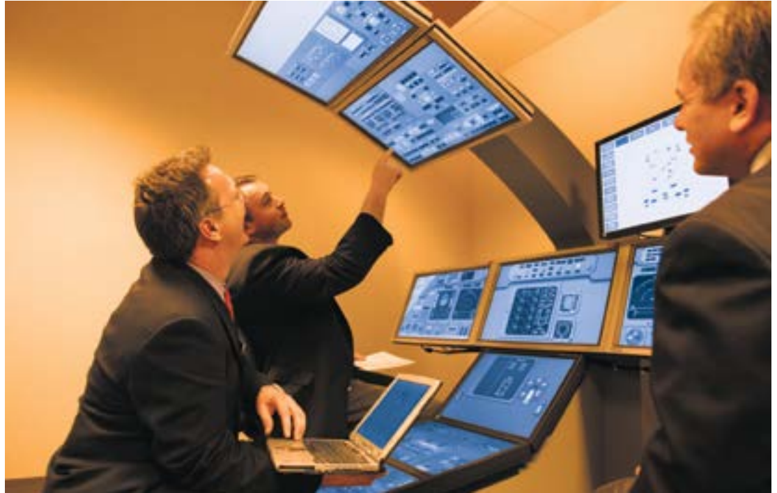
FlightSafety uses graphical flight deck simulators as a bridge between ground school and full-motion simulators. The device replicates what pilots will see in the sim, allowing them to review system schematics, checklists and lessons and practice crew resource management. In addition, students can use it as part of instructor-led or self-paced learning.
