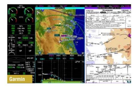
displays of efficiency. For example, range rings give an instant view of available range at current power settings. And the vertical situation display shows wind information delivered via Sirius XM, Garmin Connext via Iridium satcom or ADS-B in, helping pilots pick the best altitude while en route.
