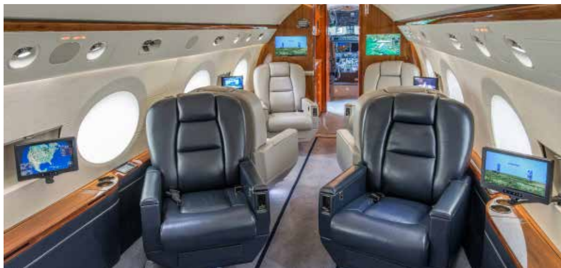
Honeywell’s Ovation touchscreen CMS lets passengers control cabin environmental conditions such as lighting, seats, temperature, galley at their seat or from a mobile electronic device.
