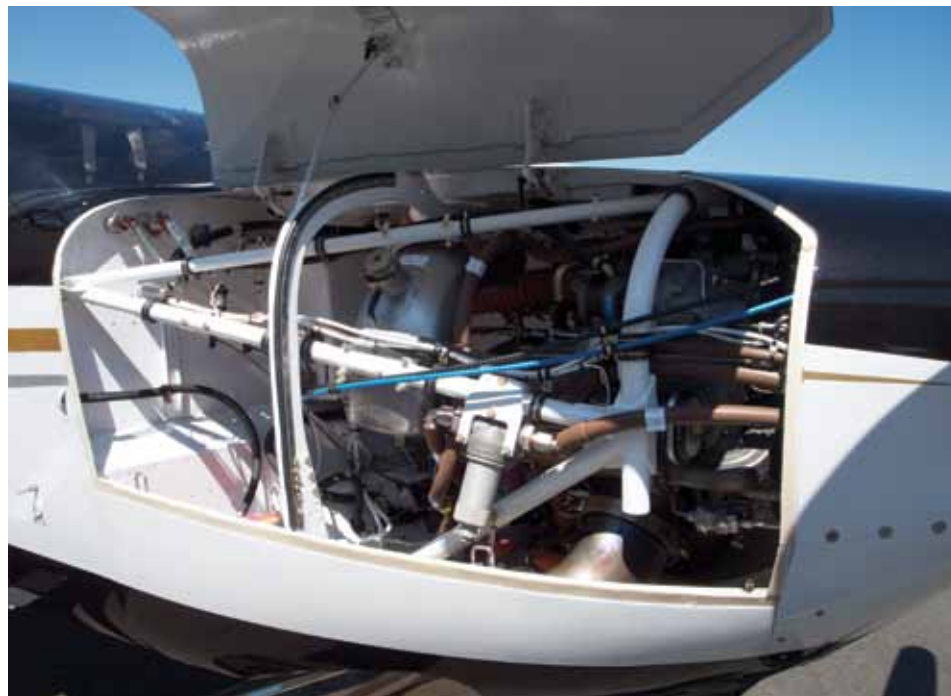
Soloy's Mark II Cessna 206 modification involves a complete firewall-forward replacement with a Rolls-Royce 250-B17F2 turboprop, a bleed-air heating system, hinged cowl and reversing propeller.
