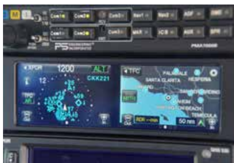
The Lynx NGT-9000 by L-3 Aviation Products combines a transponder with ADS-B OUT/IN.
