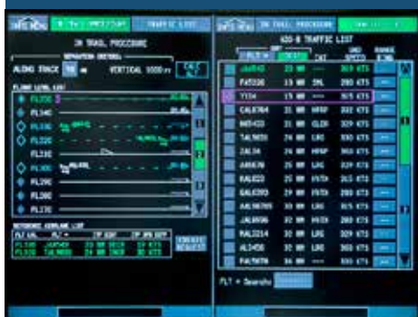
Rockwell Collins is implementing ADS-B in features, which show details about other traffic as well as employ functions such as in-trail procedures.
