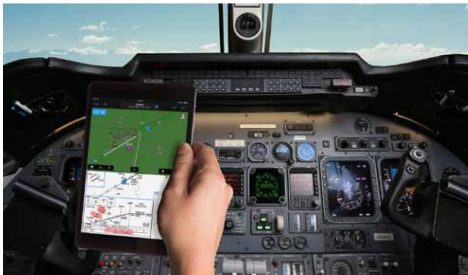
The Garmin ADS-B solution for the Learjet 60 can include ADS-B IN with installation of the Flight Stream 210.
