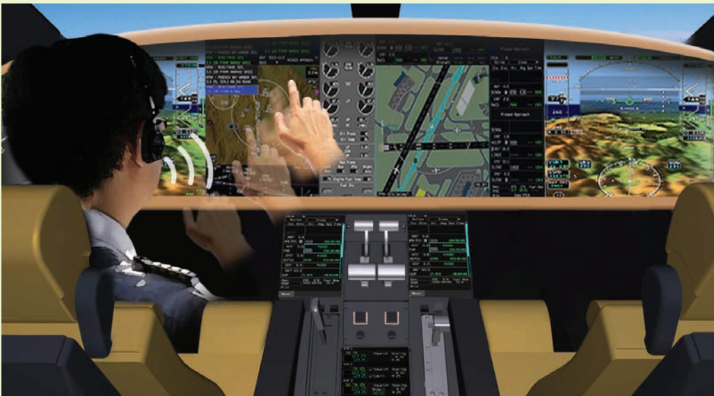
This Honeywell rendering illustrates the possibilities of future avionics. In addition to large displays that fill the panel, Honeywell foresees enhanced vision and sensing, improved pilot interface and modality options and an automated cockpit assistant contributing overall to an enhanced and more intuitive cockpit.
