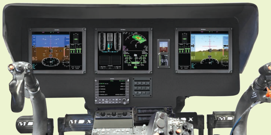
Universal Avionics is developing a fully integrated flight deck for the MD Helicopters Explorer. This mockup of the twin-engine helicopter's cockpit highlights some of Universal's unique design elements.
