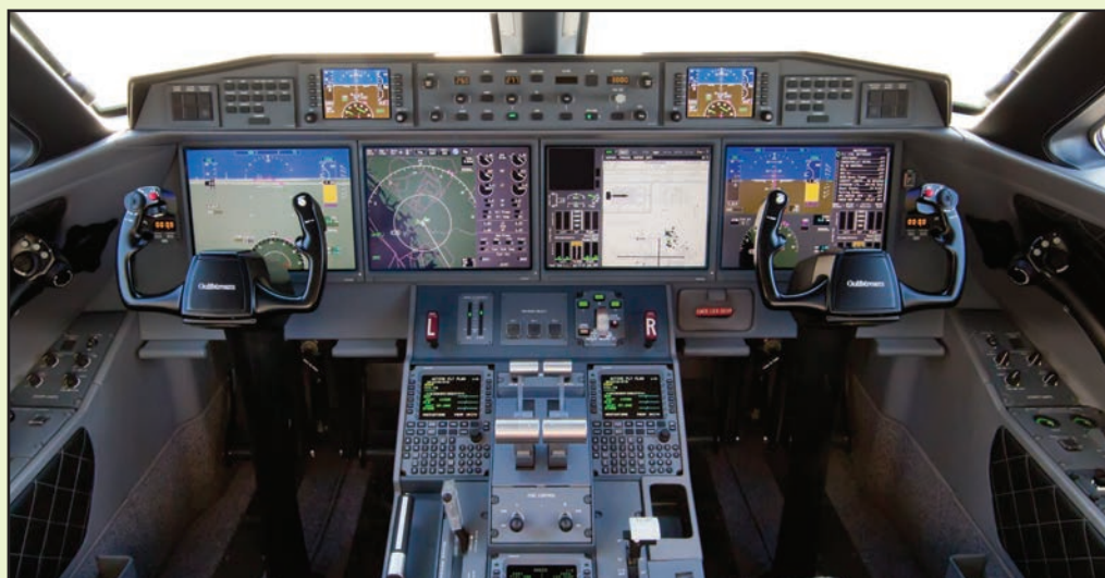
Gulfstream's PlaneView II flight deck in the G650 is the most current technology cockpit offered in a new business jet. Based on Honeywell's Primus Epic avionics, PlaneView features include EVS II infrared enhanced vision system, HUD II head-up display, synthetic vision on the primary flight displays, triplex FMS, automatic emergency descent mode and Honeywell IntuVue 3-D weather radar.
