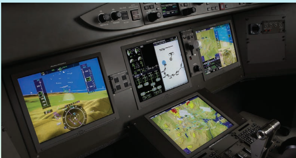
Big displays are proliferating in modern cockpits, shown here in this Rockwell Collins Pro Line Fusion flight deck. A unique feature in the Fusion synthetic vision display (which is also visible in the synthetic vision image on the associated head-up display) is the destination airport dome blooming above the compass rose.
