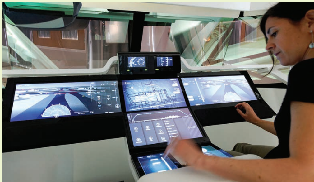
The Thales Avionics 2020 demonstrator is used to highlight capabilities that could come into play for a circa-2020 business jet flight deck. Controlled entirely by touchscreens, the Avionics 2020 design aims to preserve pilots' cognitive resources so they can focus on decision-making and not fiddling with avionics.
