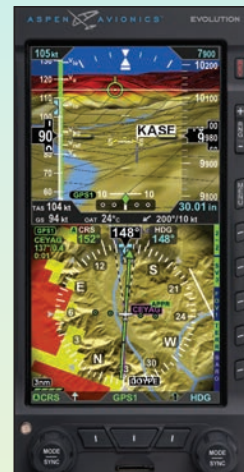
Aspen Avionics has managed to stuff an enormous amount of information into its Evolution display, which conveniently fits into two
