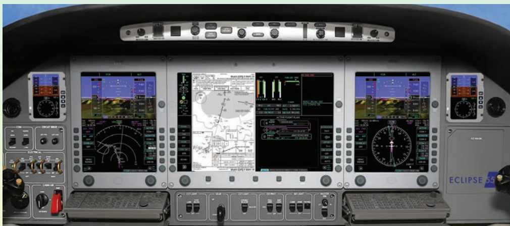
The Eclipse 550 very light jet features a fully integrated flight deck by Innovative Solutions & Support. Instead of FMS control-display units, two retractable keyboards are available for alphanumeric input.
