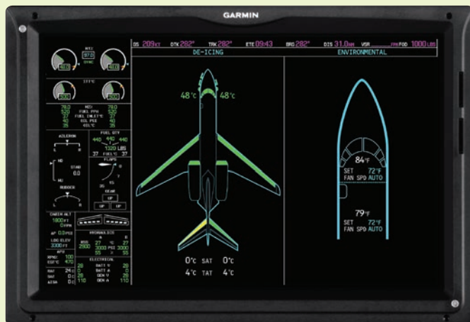
Garmin's G5000 system employs the far more intuitive icons shown above on the GTC 570 touchscreen controller. This vastly simplifies the avionics interface for pilots, who can quickly pull up information such as the synoptics chart below.
