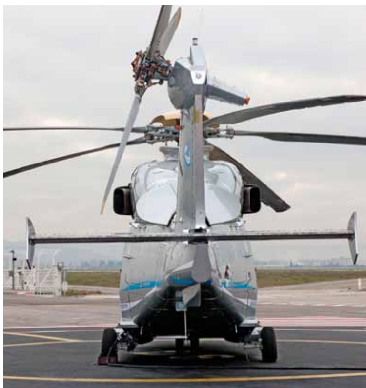
The EC-175s wide footprint gives it good stability during ground taxi. The landing gear retracts only partially up, so that the helicopter could be landed gear-up without the fuselage touching the ground.
