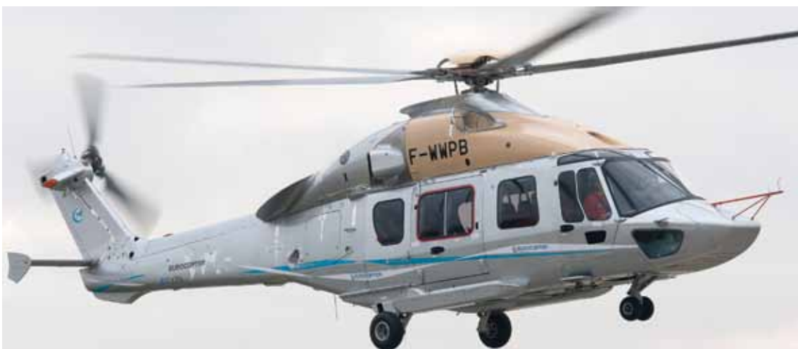
F-WWPB is the first EC175 prototype (PT1). The medium twin features a new-generation Spheriflex five-blade main rotor and three-blade tail rotor.
