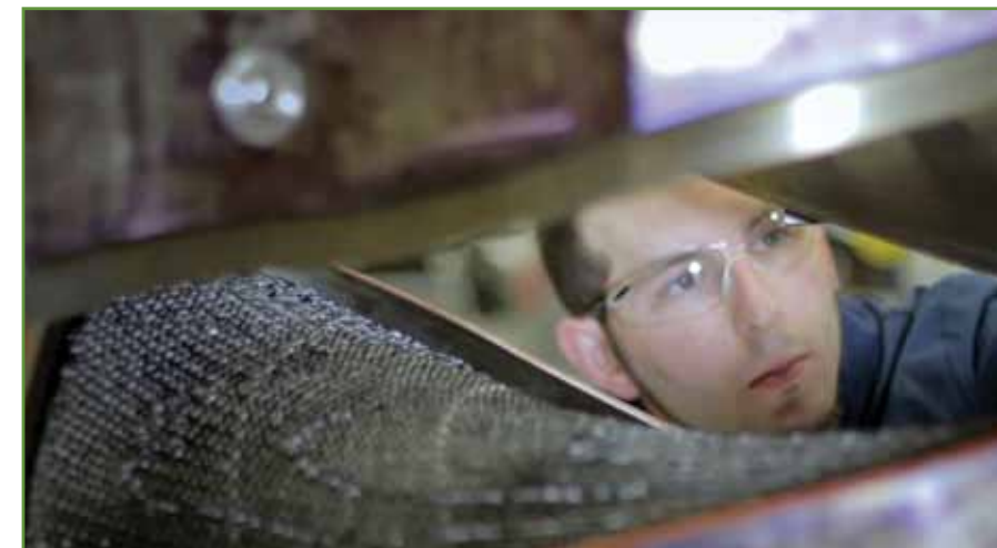
CFM is using a new 3-D woven composites process for its aero-acoustic geometry fan blades, fan case and several other parts of its Leap engine.
