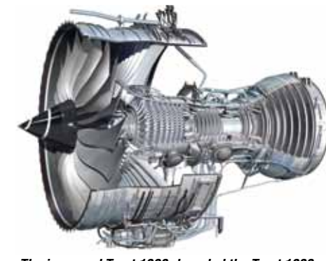
The improved Trent 1000, branded the Trent 1000-Ten, from Rolls-Royce will provide a modest but welcome one-percent increase in efficiency.
