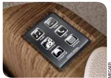
The iFeel controller includes touch-screens with customizable icons.
